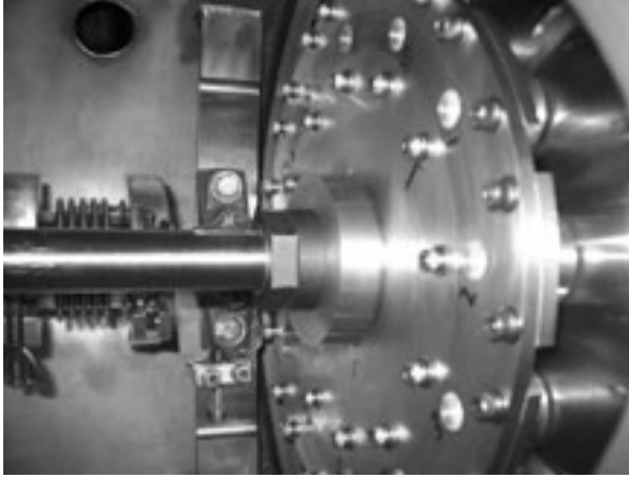
Fig. 1. Showing backside of revolver disc with sabot cups pressed against front plate.
