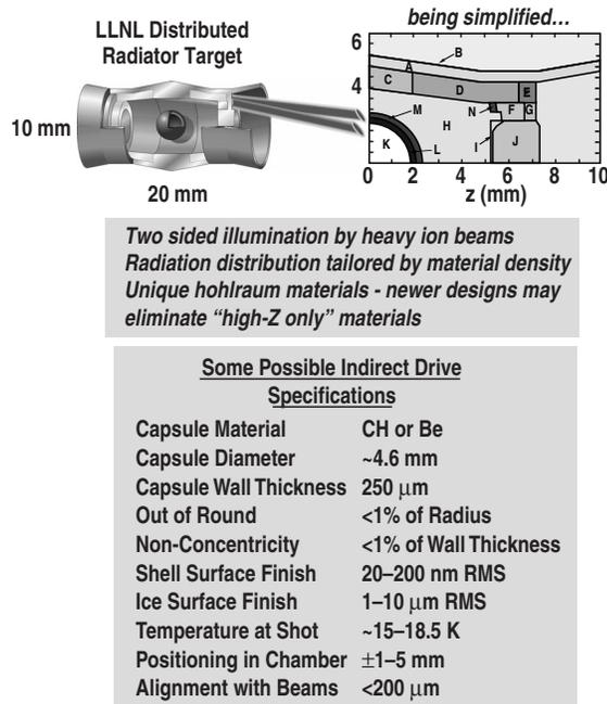
Fig. 2. LLNL distributed radiator target is driven by heavy ion beams.<sup>4</sup>
