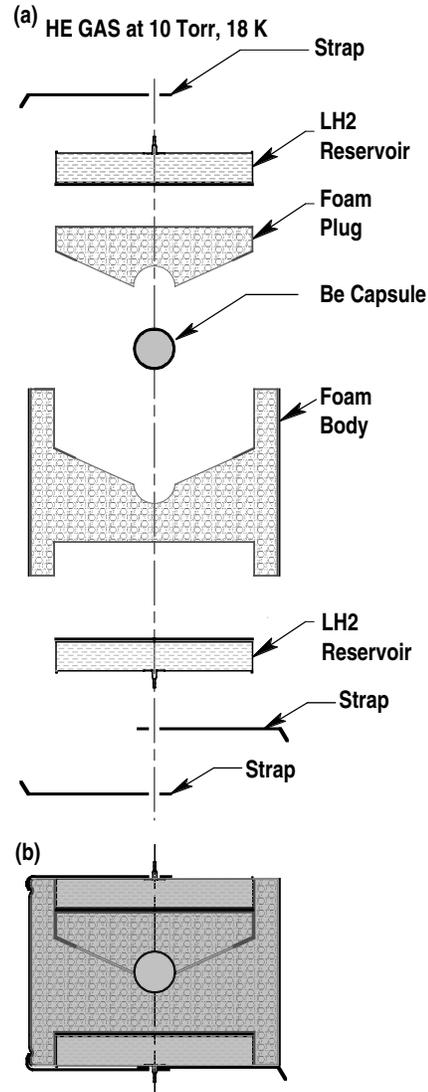
Fig. 4. (a) Components of Z-pinch target subassembly, (b) completed target subassembly.
