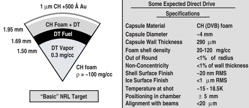
Fig. 1. Laser fusion baseline high-gain target and expected target specifications.
