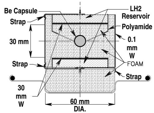
Fig. 3. Z-pinch target assembly from SNL is placed within a “dynamic hohlraum”.
