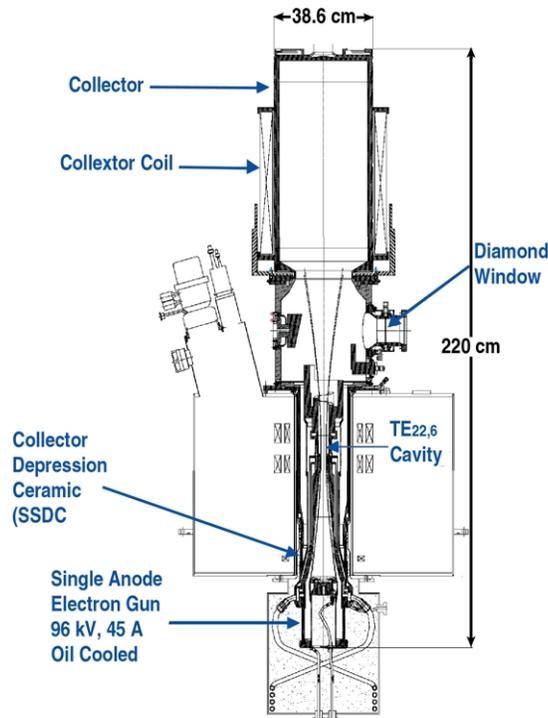
Fig. 2. Schematic view of the CPI 1.5 MW 110 GHz depressed collector gyrotron.
