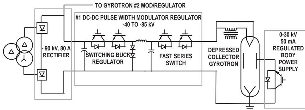
Fig. 3. Schematic of the depressed collector power supply, showing the transformer rectifier set, the pulse width modulated regulator, the fast series protection switch, and the high speed highly regulated body power supply.
