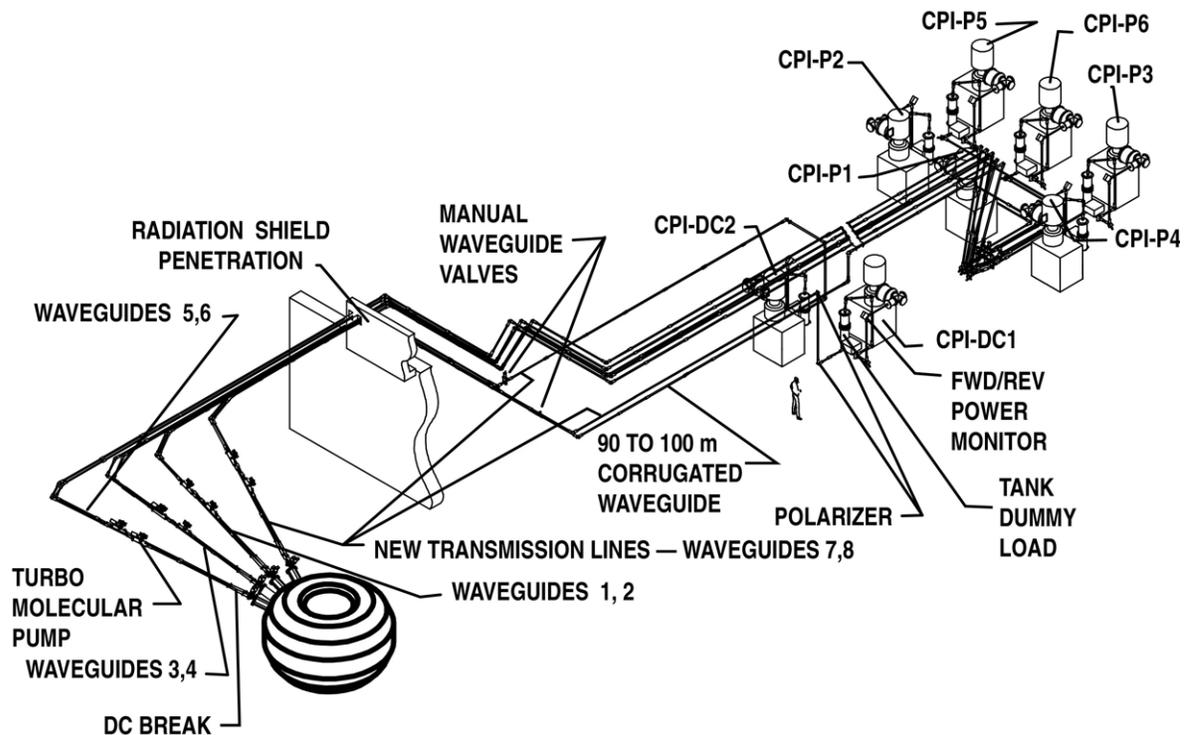
Fig. 1. Schematic of the DIII-D EC system, showing the location of the gyrotrons and the routing of the transmission lines. Key waveguide components are also identified.
