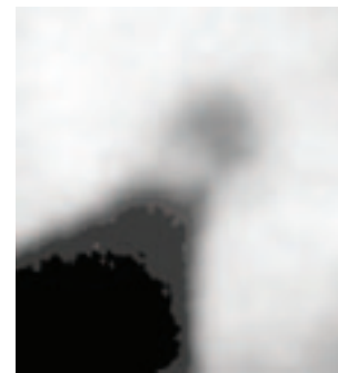
Fig. 6. Backlit image from indirect drive experiment. Because the Au density is much higher in this case, the intensity is rendered with a logarithmic scale to show both the extent of the vapor and the tendrils extending toward the collapsed shell.
