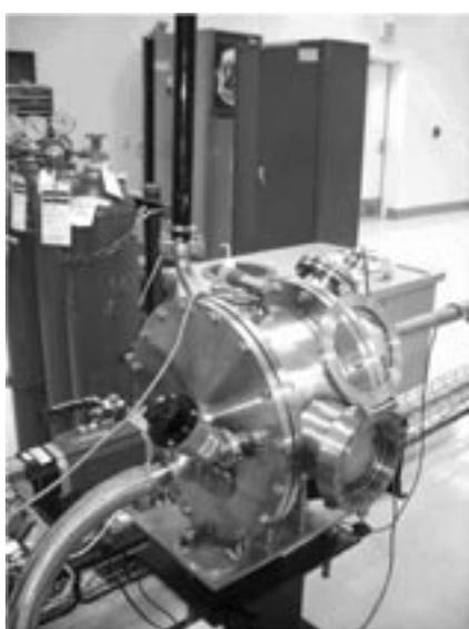
Fig. 3. Targets are loaded into the revolver chamber.
