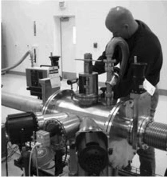
Fig. 5. Sabot deflector with light sources and camera.
