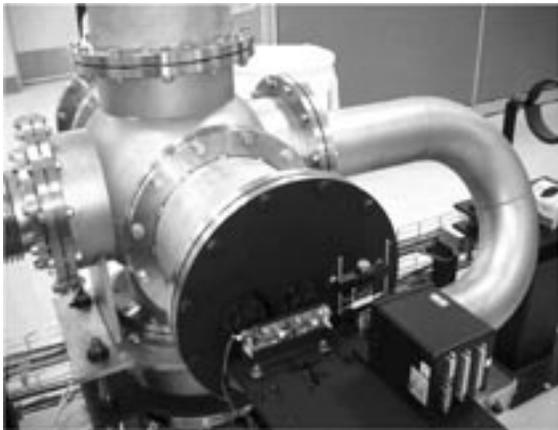
Fig. 7. Target tracking detectors use photodiodes for timing and a line scan camera for position measurement.
