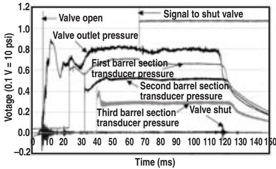
Fig. 8. Sensor output vs time for a Garolite shot.
