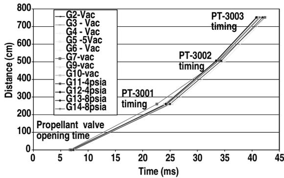
Fig. 9. Projectile position vs time for several Garolite shots (initial target position is 0.54 m).
