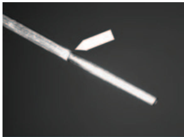
Fig. 7. Inner self-centering needle showing the square centering fins (~0.05 inch diameter).
