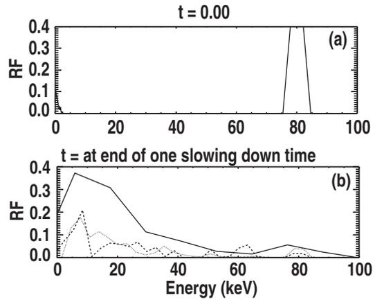
**Figure 2.** Distribution of energetic ions from NB energetic ions by ICRF.
