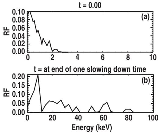
**Figure 1.** Distribution of energetic ions excited from thermal ions by ICRF.
