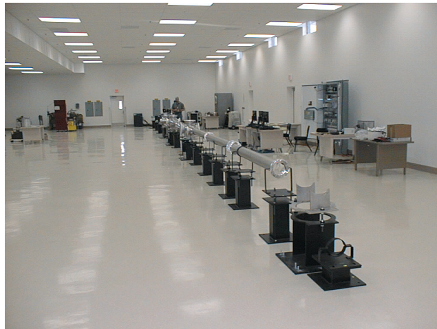
Figure 1. A gas gun for launching inertial fusion energy targets.
