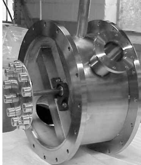
Fig. 3. Revolver target loading assembly is part of the revolver chamber
