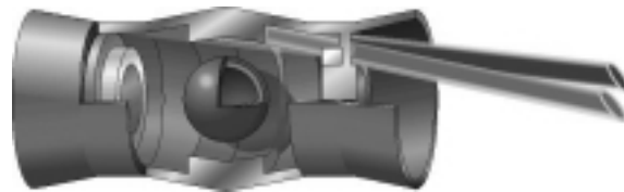
Fig. 2. Heavy-ion driven indirect drive target for IFE designed at LLNL [2]. The length of the target is 20 mm and the average radius is \sim 5\ \text{mm} . The central fuel capsule is \sim 4.7\ \text{mm} in diameter and consists of an ablator (capsule) surrounding a solid DT fuel layer of 0.32 mm thickness.
