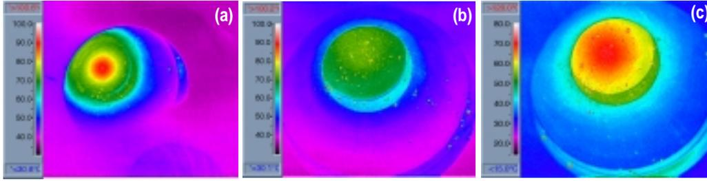
Fig. 1. The infrared images of the gyrotrons windows differ qualitatively. In (a) the CPI-P2 window infrared image is seen to have a Gaussian character with several pinpoint hot spots. (b) The CPI-P3 window has a much broader temperature, which is nearly flat across the central part of the image. (c) The infrared image has a distinctive hot area in the middle of the window similar to CPI-P2, although the parameters of the diamond disk are similar to the CPI-P3 window.
