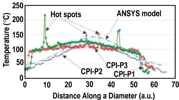
Fig. 2. Temperature profiles for the three CVD diamond windows measured with an infrared camera are compared with the ANSYS calculation for one of them. The measurements are broader and lower than the model.
