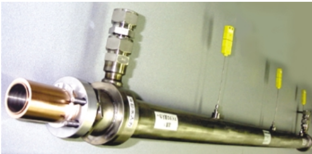
Fig. 1. 110 GHz 1 MW load (attenuator) in 31.75 mm corrugated waveguide with stainless steel water jacket.
