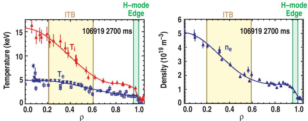
Fig. 2. Clear double barriers are seen in the ion temperature and the electron density, but not in the electron temperature in this shot.
