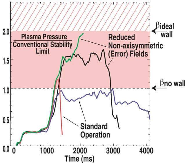
Fig. 4. Plasma pressure is stably maintained up to the ideal wall limit, which is a factor two above the conventional pressure limit, with stabilization of the resistive wall mode. The nonaxisymmetric error fields are reduced by continued plasma rotation.
