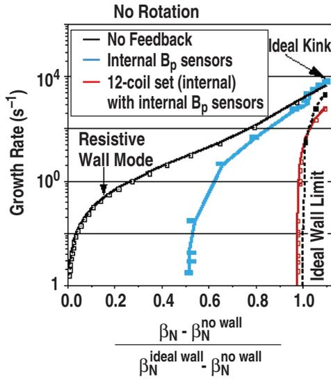
Fig. 5. With internal sensor the obtainable  $\beta_N$  is halfway between the no-wall limit and ideal wall limit. With twelve internal control coils the obtainable value is very close to the ideal wall limit.
