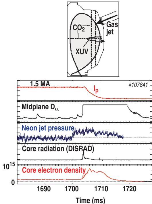
Fig. 6. Disruption mitigations in DIII-D. A high pressure gas jet is injected into the plasma. The plasma current has a smooth decay, and the gas is seen reaching the center of the plasma from the radiation and density measurements.
