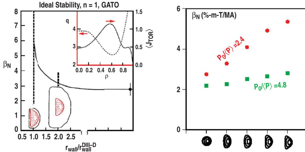
Fig. 3. Calculation with the code GATO shows that  $\beta_N = 6$  can be obtained with tight fitting wall where as the limit is much lower with the walls far from the plasma. Higher  $\beta_N$  can be obtained with higher triangularity and broader pressure profiles.
