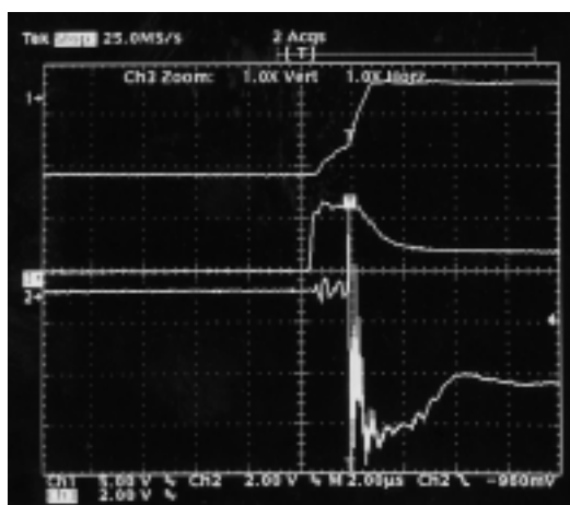
Fig. 2. Results of the crowbar wire test in which a 36 gauge wire survived repeated trials. The middle trace is the wire current (400 A/div), the bottom trace is the crowbar current (400 A/div), and the top trace is the output voltage.
