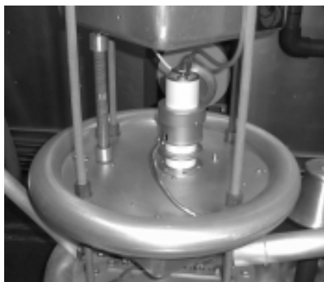
Figure 2. Photograph of a single stage of the crowbar switch assembly.
