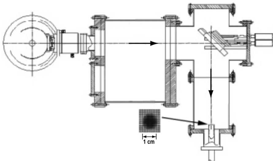
Fig. 3. The single mirror coupling scheme is presented along with the footprint of the beam on thermally sensitive paper at the waveguide input.
