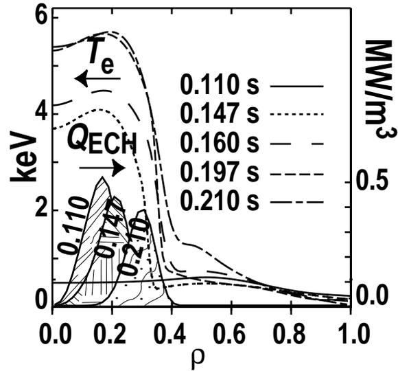
Fig. 5. An electron temperature profile is shown in which the transport barrier was formed by application of ECCD early in the development of the discharge.
