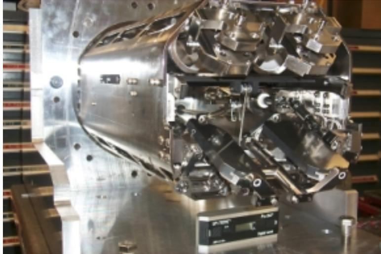
Fig. 2. The articulating launcher, developed by the Princeton Plasma Physics Laboratory.
