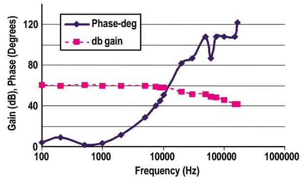
Fig. 4. The open-loop frequency response of the MFTF grid driver amplifier prior to its modification.
