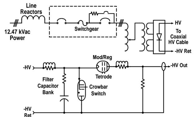
Fig. 1. A single-line illustration of the ECH power system.
