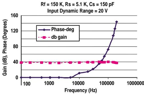
Fig. 5. The response of the grid driver amplifier modified with feedback.
