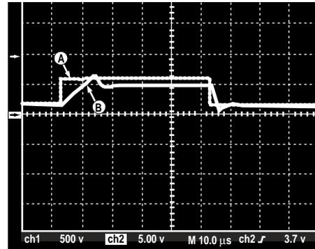
Fig. 6. The large signal response of the modified grid driver amplifier to a 10 kHz square wave. Trace “A” is the input signal (5 V/div). Trace “B” is the amplifier output (500 V/div).
