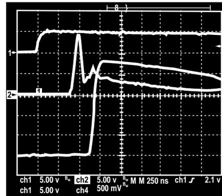
Fig. 2. Triggering tests of a single stage of the crowbar switch system. The top trace is the input fire command; the middle trace is the trigger grid voltage (500 V/div); the bottom trace is the discharge current through the HX-2500 (100 A/div). The horizontal scale is 250 ns/div.
