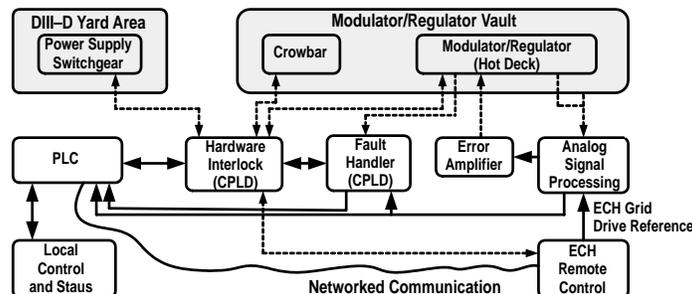
Fig. 7. The ECH power system controls architecture. The dashed lines indicate signals transmitted over fiber-optic links.
