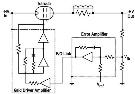
Fig. 3. A simplified schematic diagram of the M/R illustrating the essential components of the feedback loop.
