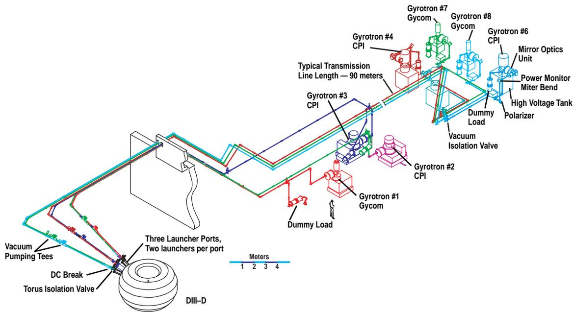
Fig. 1. DIII-D 110 GHz ECH transmission systems.
