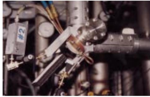
Fig. 2. 1.25 in. power monitor miter bend with water-cooled, GlidCop mirror.
