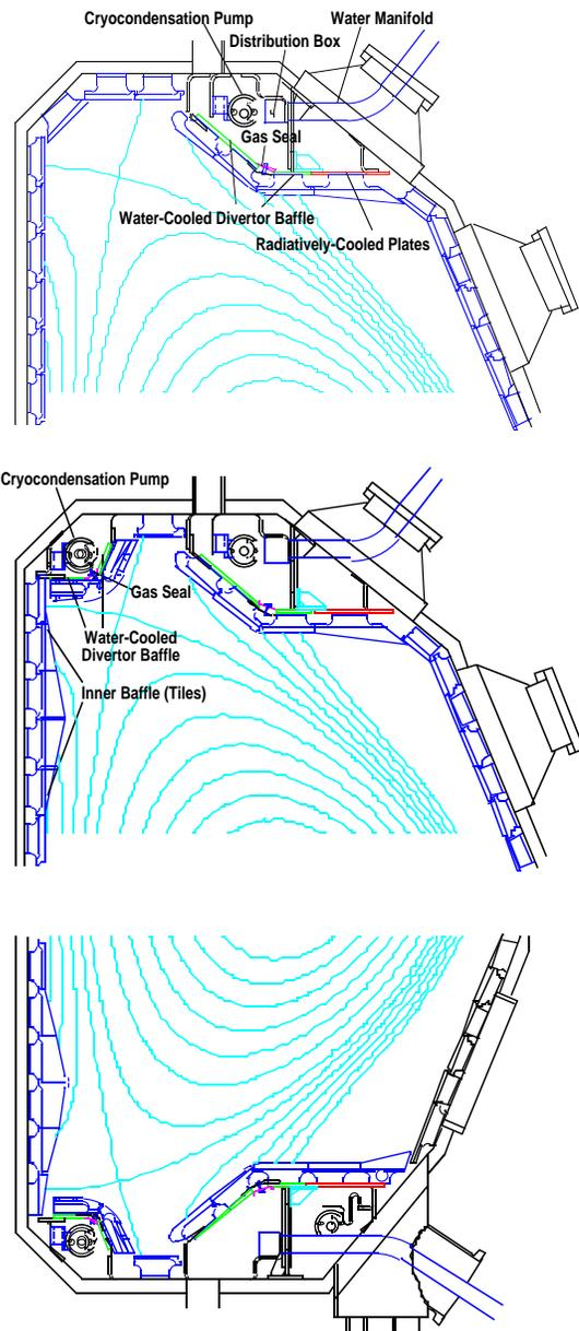
Fig. 4. Phased approach to the RDP installation. (a) Phase 1A installed 1997, (b) Phase 1B adds private flux baffle, and (c) Phase 1C adds inner and outer lower baffle structures.
