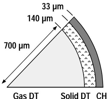
Fig. 1. Direct drive target for GEKKO XII Upgrade
