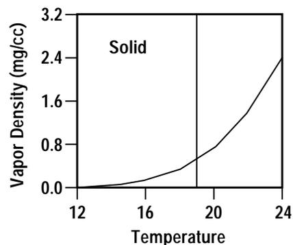
Fig. 4. Temperature/density diagram for cryogenic targets.
