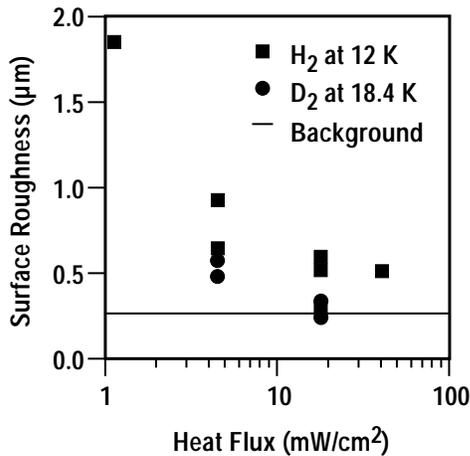
Fig. 6. Surface roughness vs. heat flux. Beta heating in 100  $\mu\text{m}$  DT is  $\sim 0.5 \text{ mW/cm}^2$
