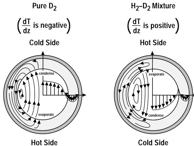
Fig. 7. Thermal gradient layering diagrams
