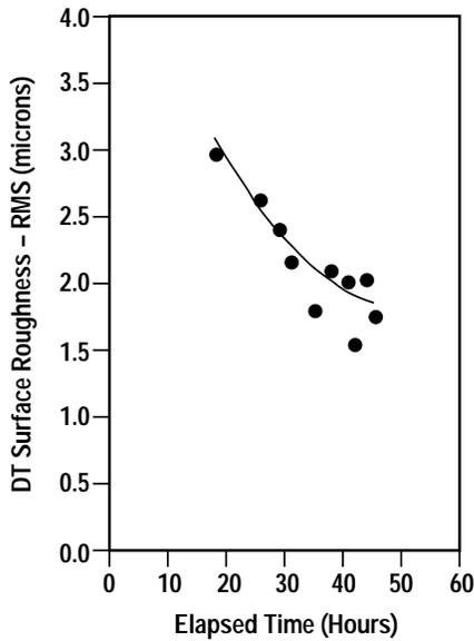
Fig. 5. Beta layering uniformity vs. time.
