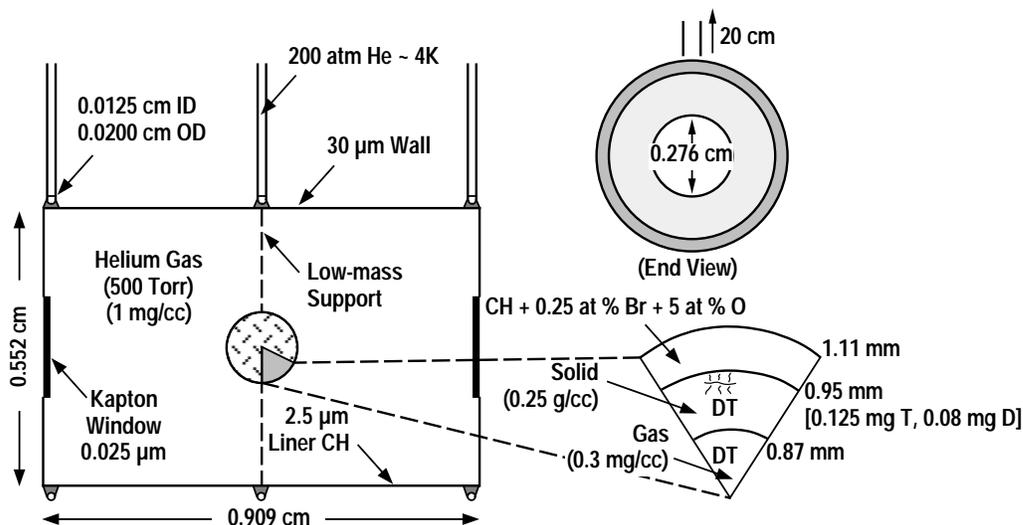
Fig. 2 . An indirect drive target for NIF
