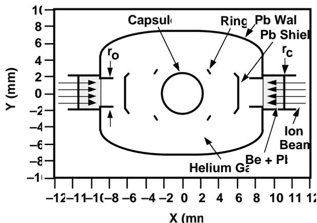
Fig. 9. HIB target for inertial fusion energy application
