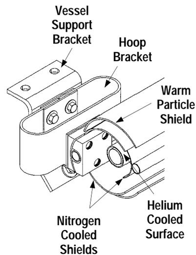
Fig. 3. Cryopump cross section and support structure
