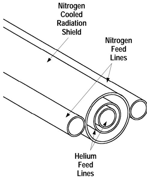
Fig. 4. Helium and nitrogen cryopump feedline configuration
