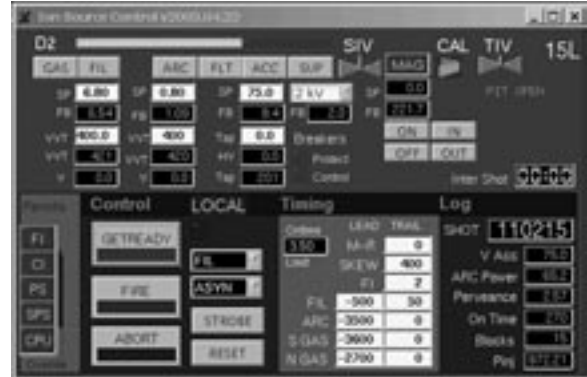
Fig. 1. An example of a Kylix generated GUI — the beam operator's console.
