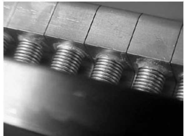
Fig. 6. Successful Palcusil-10 braze of replacement bellows into an ex-service source grid rail module.
