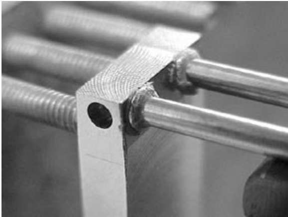
Fig. 7. Grid rail to holder joint packed with Palcusil-25 braze wire and paste prior to braze test.
