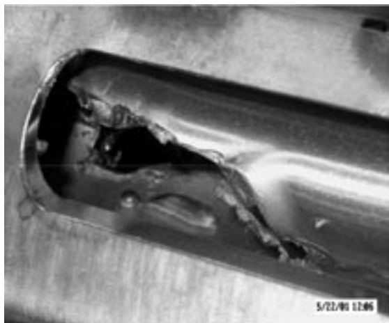
Fig. 3. Damage of waveguide due to ECH shot with shutter closed.
