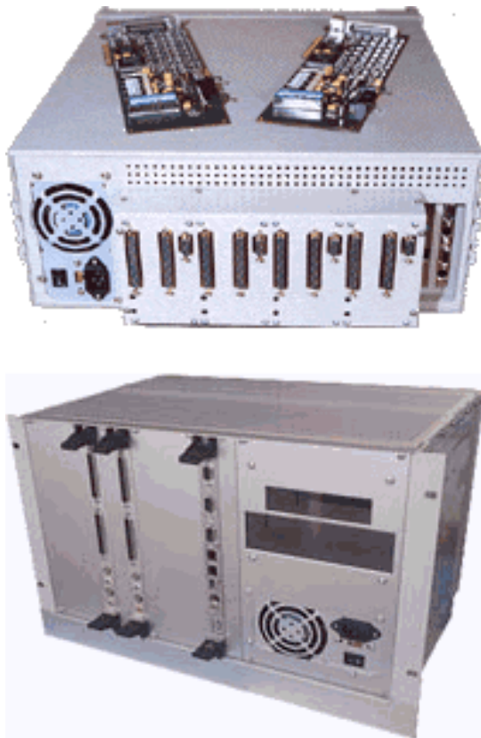
Fig. 1. PCI (top) and cPCI (bottom) data acquisition systems. (Images printed with permission of D-TACQ Solutions Ltd.)
