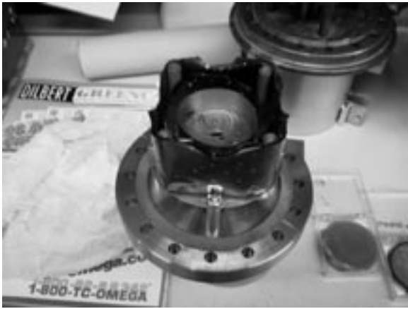
Fig. 2. Lithium source flange showing spiral tungsten filament and tantalum heat shielding. The filament, biased -1300 VDC below the lithium source (seen at right), electron heats the source to 1200^{\circ}\text{C} .
