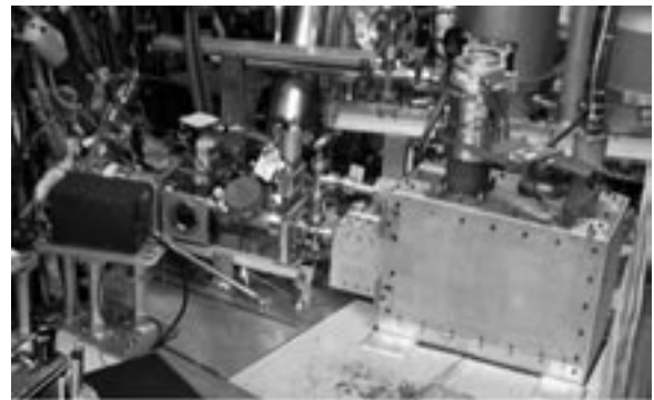
Fig. 1. Above, the DIII-D lithium beam's lithium ion gun and accelerator, electrostatic lens, and sodium vapor neutralizer, all enclosed behind magnetic shielding (below at right), seen as installed on the DIII-D tokamak at General Atomics.
