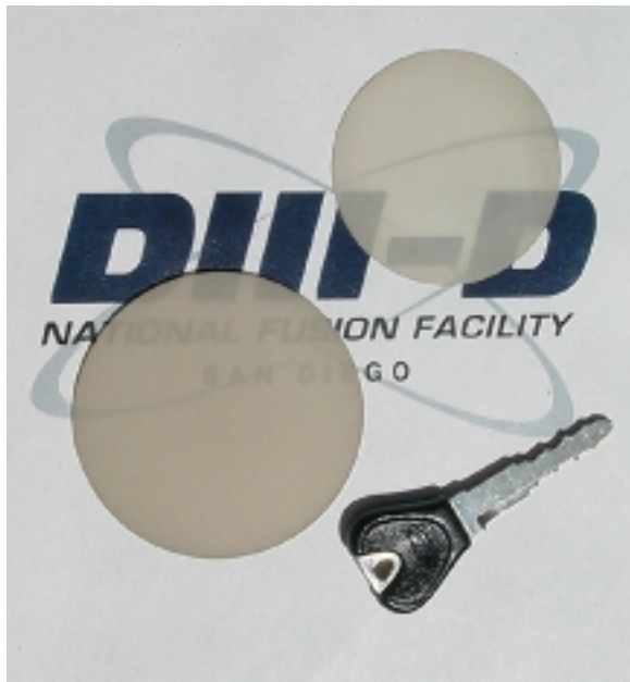
Fig. 6. Photograph of two CVD diamond disks. The smaller has diameter 60 mm and thickness 0.55 mm. The larger is 73 mm diameter and 1.7 mm thick. Typical loss tangents at 110 GHz are < 5 \times 10^{-5} for these disks.
