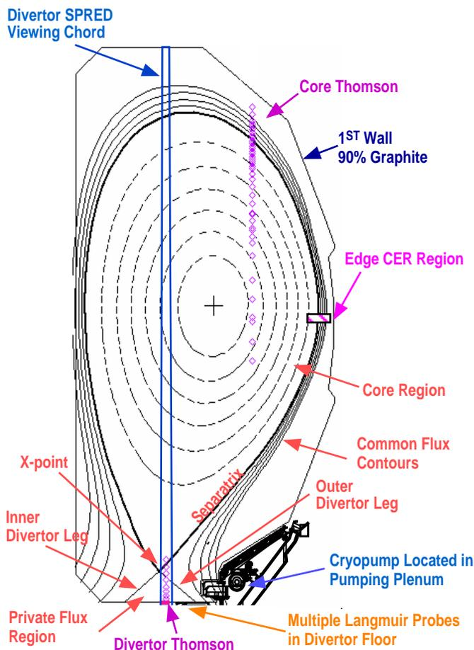
Fig. 1. A cross section of the DIII-D vacuum vessel with a flux contour plot of a typical lower single-null diverted plasma configuration is shown along with the locations of important divertor diagnostics. Also shown are the inner and outer divertor leg locations, the common and private flux regions, and the pumping plenum and cryo-pump.
