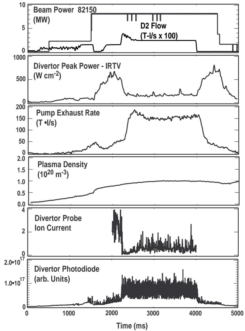
Fig. 2. The time history of several important discharge parameters from DIII-D discharge # 82150, where D<sub>2</sub> gas puffing combined deuterium exhaust using the cryo-pump was used to reduce the peak heat flux to the divertor by a factor of five compared to pre-puff conditions. The low heat flux condition was maintained in nearly steady-state for about 2 s.
