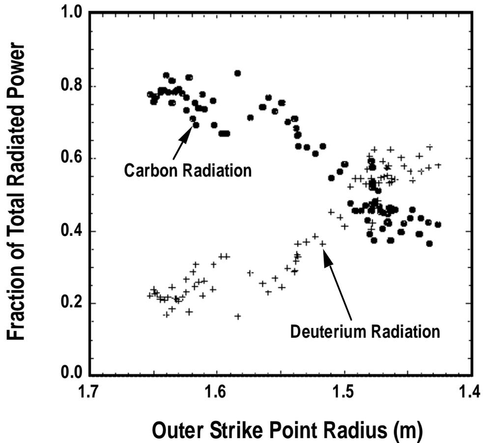
Fig. 5. The fraction of the total radiated power due to carbon and deuterium along a vertical chord viewing the divertor at  $R = 1.48$  m is shown as a function of the location of the outer strike point during a strike point sweep. The line integrated radiated power due to carbon and deuterium are obtained from VUV spectroscopy as described in the text, and the total radiated power is obtained from bolometry.
