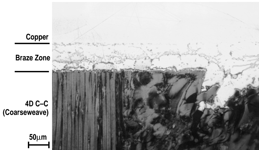
Fig. 3. Microstructure of cross-sectioned braze joint; braze alloy (Copper ABA) between coupons of OF Copper UNS-C10100 and CFC, type FMI 4-D C-C Coarseweave composite. *Interface phase of TiC (~5 \mu\text{m} thickness) formed during brazing. NOTE: Z-axis fibers are perpendicular to braze plane.
