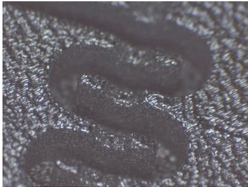
Fig. 3. A magnified view of the serpentine portion of the waveguide circuit.
