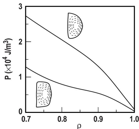
Fig. 1. Comparison of edge pressure of a high squareness discharge to that of a moderate squareness discharge.
