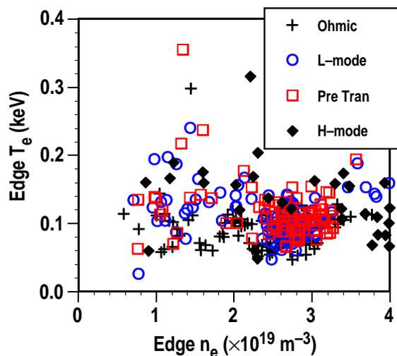
Fig. 1.  $T_e$  versus  $n_e$  evaluated the the  $n_e$  pedestal.
