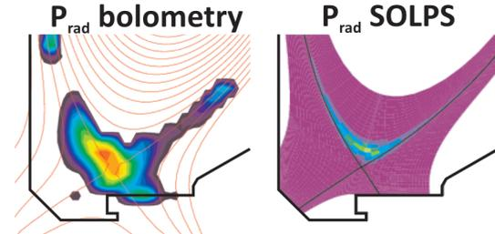
Figure 3: Modeling of radiated power in He plasma.
