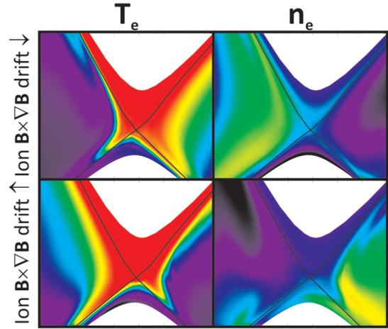
Figure 2: UEDGE modeling of low density H-mode in forward (top) and reverse (bottom)  $\mathbf{B}_T$  in DIII-D.
