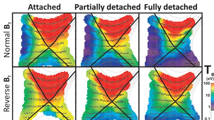
Figure 1: Electron temperature measured by DTS in forward (top) and reverse (bottom)  $B_T$  in the transition to divertor detachment.
