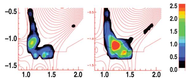
Fig. 2. Divertor radiated power distribution in the attached SF-plus ( $n_e=5 \times 10^{19} \text{ m}^{-3}$ ) and radiative SF-plus ( $n_e=7.3 \times 10^{19} \text{ m}^{-3}$ ).
