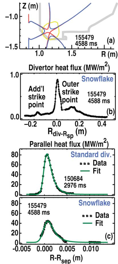
Fig. 1. (a) Near-exact SF configuration, with a contour around the X-point region showing the extent of low  $|B_p/B_{pml}| = 0.10$  region, where the poloidal magnetic field  $B_p$  is normalized to its midplane  $B_{pml}$  value, (b) divertor heat flux profile, (c) Parallel heat flux  $q_{||}$  profile projected to midplane, and the Eich function fit, for the standard and SF configurations.
