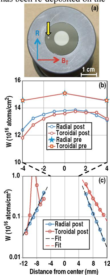
Fig. 2. Pre-exposure photograph (a); pre- and post-exposure RBS measurements of W coverage on the sample (b,c).
