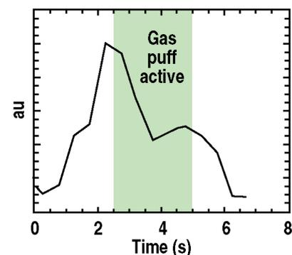
Fig. 1. MoI radiation at 386.3 nm measured by MDS spectrometer in a discharge with  $^{13}\text{CH}_4$  gas injection in L-mode.
