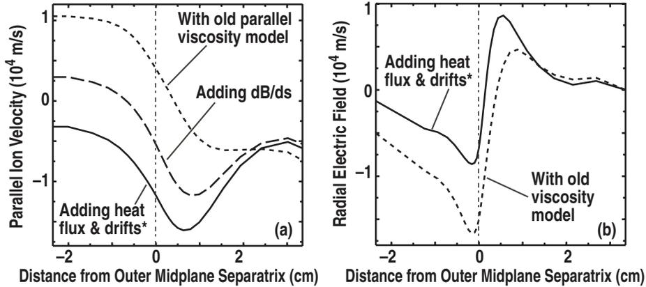
FIG. 4. Hydrogen ion parallel velocity from UEDGE for different viscosity models and the radial electric field profiles corresponding to two cases.
