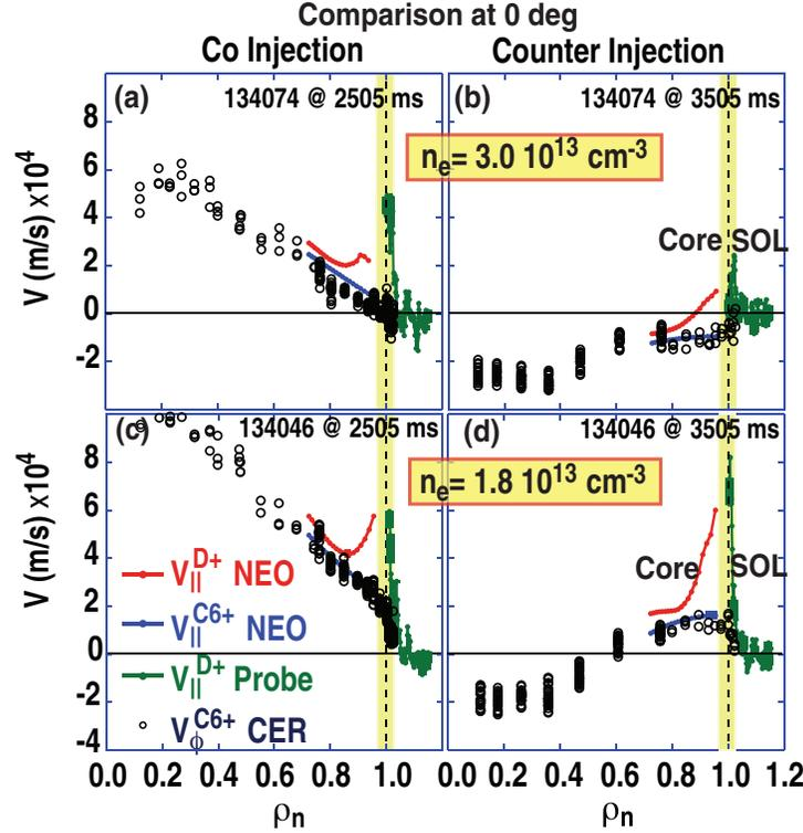
FIG. 1. Velocity comparison of the CER toroidal carbon measurement (open circles), NEO parallel carbon calculations (blue lines), NEO parallel deuterium calculations (red lines), and Mach-probe parallel deuterium measurements (green lines) for (a,c) co- and (b,d) counter-NBI injected phases versus  $\rho_n$ , the normalized toroidal flux.
