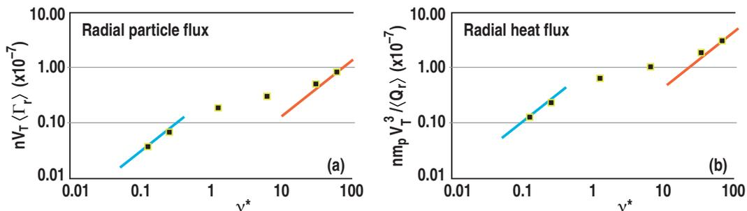
FIG. 3. COGENT simulations (dots) of the radial neoclassical ion particle flux and energy flux versus the normalized collision frequency for the case of the Lorentz collision operator. The red and blue lines correspond to analytical calculations<sup>16</sup> in the banana and Pfirsch-Schluter regimes, correspondingly. The parameters of the simulation correspond to circular geometry with  $q=3$ ,  $\epsilon=0.1$ ,  $R_0=45.6$  m,  $B_0=7.5$  T,  $T_i=3$  keV, and  $R_0/L_n=R_0/L_T=10$ .
