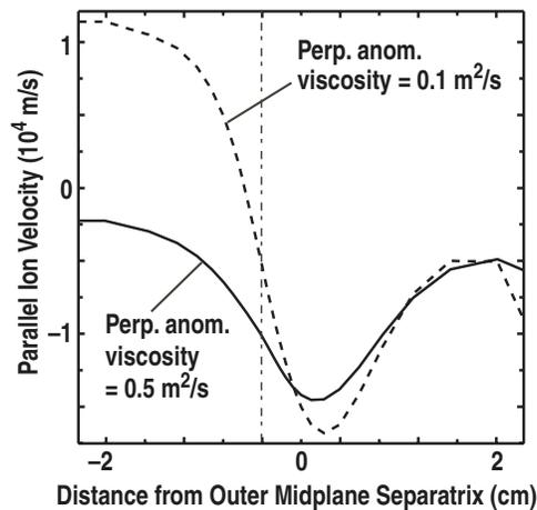
FIG. 5. The deuterium parallel velocity from UEDGE at the outer midplane for the initial case comparing anomalous parallel viscous diffusivity of  $0.5 \text{ m}^2/\text{s}$  and  $0.1 \text{ m}^2/\text{s}$ .
