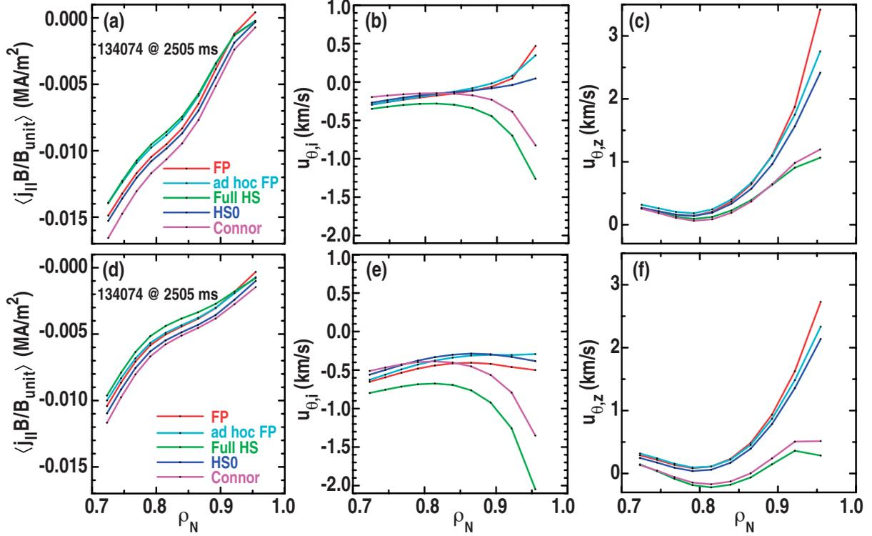
FIG. 2. Bootstrap current and deuterium and carbon poloidal flows for DIII-D #1374074 @ 2505 ms (top plots) and DIII-D #134046 @ 2505 ms (bottom plots) computed with NEO. Results from various model collision operators are compared with results from the full Fokker-Planck collision operator (FP).
