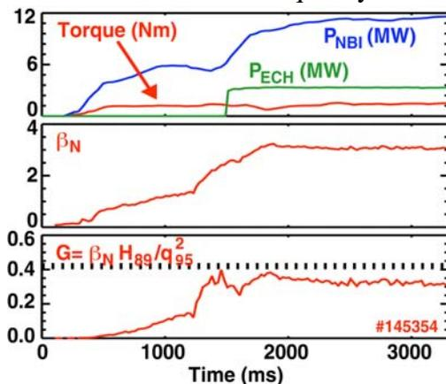
Fig. 1. Plasma shot illustrating high normalized fusion performance  $G \sim 0.35$  achieved with low torque startup.
