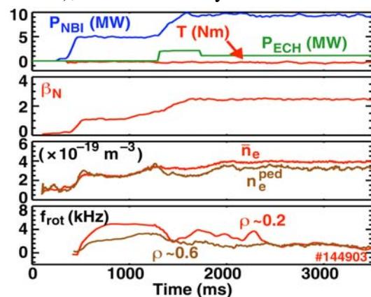
Fig. 2. Advanced inductive discharge produced and sustained with zero net torque at  $\beta_N \sim 2.4$  and rotation  $\sim 1$  kHz.
