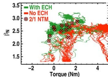
Fig. 3. Trajectories highlight the difficulty in accessing high  $\beta_N$  low torque plasmas without ECH.
