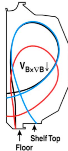
Fig. 1. The 3 principal plasma cross-sections: 1. R_{\text{TAR}} = 1.20 m, I_p = 40 m (black), 2. R_{\text{TAR}} = 1.20 m, I_p = 32 m (red), and 3. R_{\text{TAR}} = 1.66 m, I_p = 35 m (blue).
