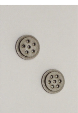
W-buttons with 1 mm dia. indents
