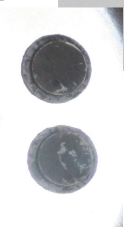
W-buttons filled with Si
