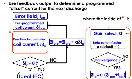
A relaxation factor is introduced to improve the numerical convergence to the desired EFC level
