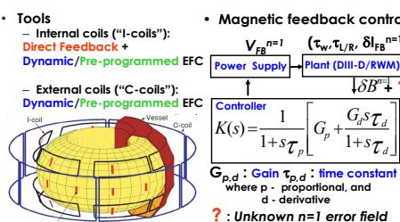
Simultaneous operation of DEFC and DF helps us to determine the necessary EFC using the feedback-stabilized RWM
