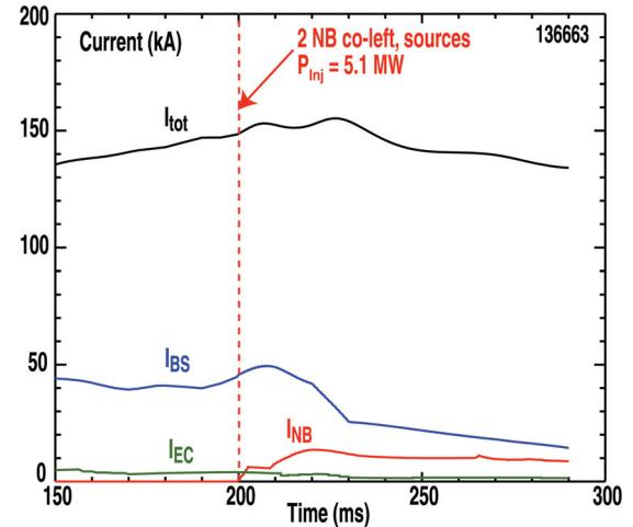
**FIG. 6.** Calculated current drive partitioning of the solenoid-free discharge 136663 with 2 co-left NB sources injected between 200-360 ms with total injected power of  $\sim 5$  MW. Based on ONETWO [27] with ion beam diffusion of  $10 \text{ m/s}^2$ , set to match experimental stored energy and neutron emission rate.
