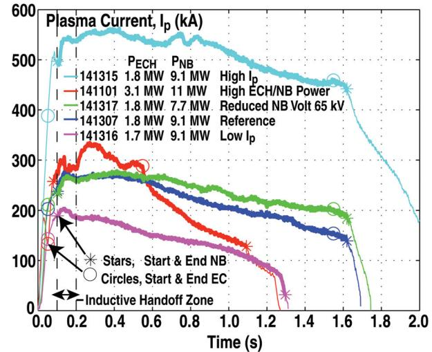
*FIG. 7. Plasma current time history for a number of discharges using a conventional (E-coil) startup of DIII-D. The E-coil is used to initiate the discharge with its current frozen in the “inductive handoff zone” (100–200 ms). Various curves show some of the major parameters varied during the campaign. Circles and stars demarcate the beginning and end of the EC and NB power phases of the discharge, respectively. The heavy portions of the line further highlight the NB phase.*
