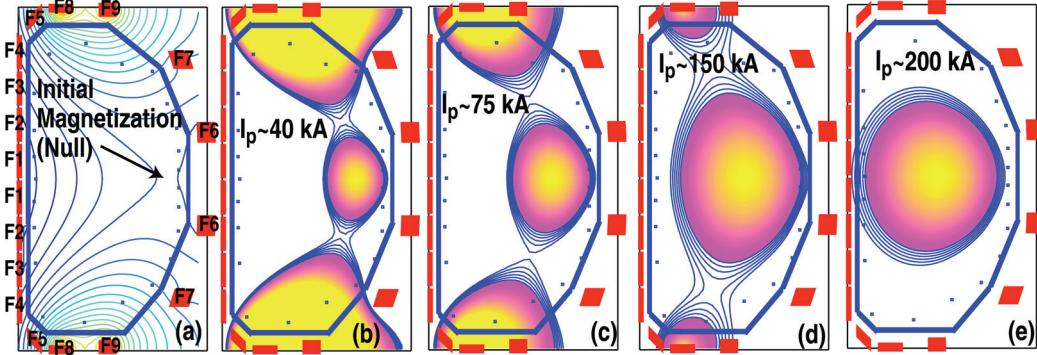
*FIG. 2. Solenoid-free scenario development equilibrium flux plots (Fiesta). Frame (a) shows the IM null formation state prior to plasma initiation. (b-e) The evolution of plasma current transfer from the PF coils with (e) the final maximum plasma current state.*
