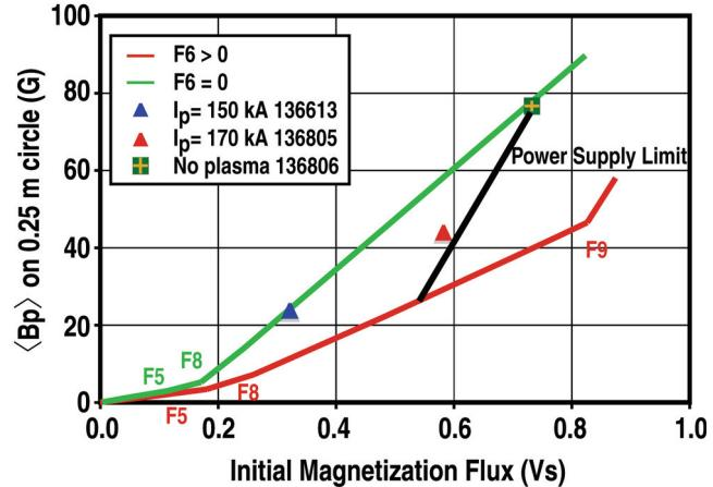
FIG. 3. Calculation of DIII-D solenoid-free IM central flux versus average stray field on the breakdown circle (Fig. 1) under ideal conditions. Two curves represent maximum flux per unit stray field for different conditions imposed on  $F6$  coil current: red for  $F6 > 0$  and green  $F6 = 0$ . Operation below these curves is not possible. Current limits (color coded) are shown along the curves. The IM states for several discharges are shown along with limits imposed by the PS system.
