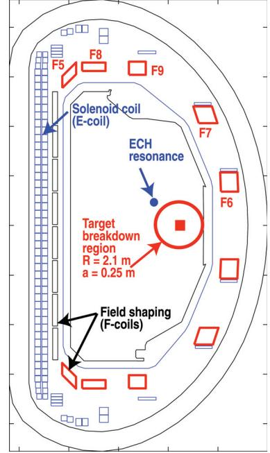
*FIG. 1. DIII-D cross-section showing major axisymmetric magnet systems. The PF coil system is composed of the E- and F-coil systems and is used for normal plasma initiation. For solenoid-free startup, only coils F5–9 (above/below the midplane) are used for plasma initiation. Circle represents the plasma target. The ECH resonance is shown.*
