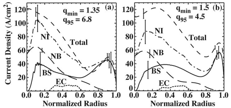
Fig. 3. Radial profiles of the current density components. (a)  $q_{min} = 1.35$ ,  $q_{95} = 6.8$ ,  $\beta_N = 3.6$ , (b)  $q_{min} = 1.5$ ,  $q_{95} = 4.5$ ,  $\beta_N = 3.45$ . The total current density is from an experimental equilibrium reconstruction, the noninductive current density components are calculated from models [bootstrap current (solid), neutral beam driven (long-dash), electron cyclotron driven (dot-dot-dot), total noninductive (dot-dash)].
