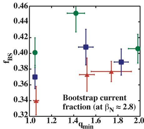
Fig. 2. Bootstrap current fraction at  $\beta_{\text{N}} = 2.8$  as a function of  $q_{95}$ , 4.5 (red triangles), 5.6 (blue squares), 6.8 (green circles), and  $q_{\text{min}}$ .
