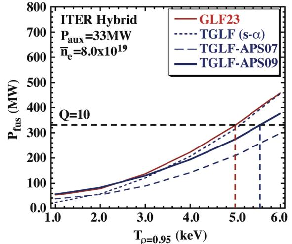
Fig. 2. Predicted fusion power versus pedestal temperature at fixed density for an ITER hybrid case with a flat density profile using the TGLF (blue) and GLF23 (red) models.
