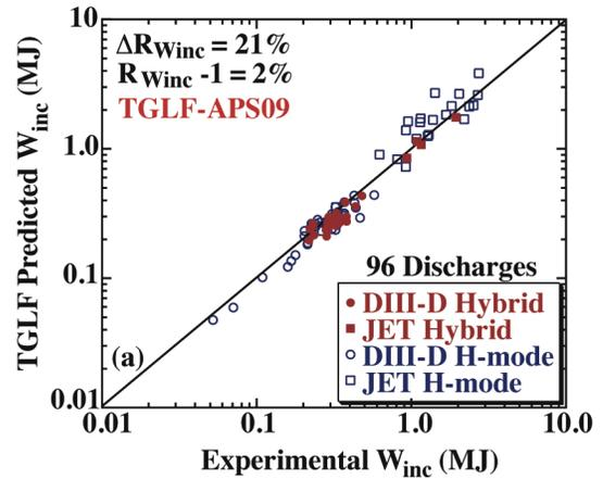
Fig. 1. Predicted incremental stored energy  $W_{inc}$  using TGLF-APS09 versus experimental  $W_{inc}$  for 30 DIII-D hybrids, 4 JET hybrids, 40 DIII-D H-modes, and 22 JET H-mode discharges.
