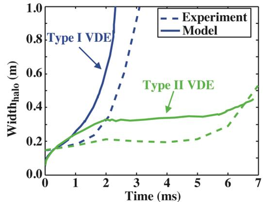
Fig. 1. Halo width vs time after first contact with vessel wall. Dashed lines are experimental JFIT reconstruction values, solid lines are model results. Type I VDE (blue), Type II VDE (green).
