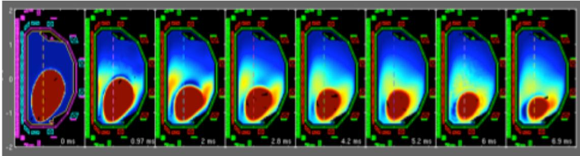
Fig. 3. Simulation of current density evolution during Type II VDE #93204.
