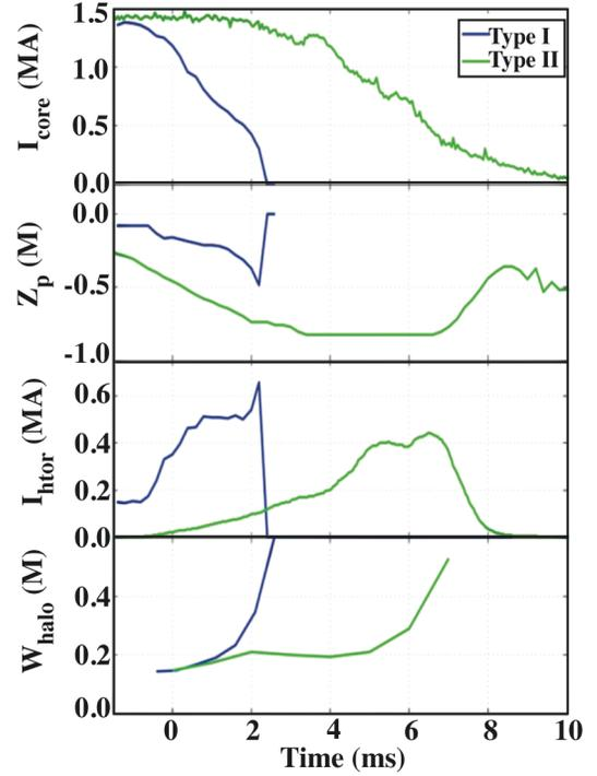
Fig. 2. Comparison of Type I (blue) #110216 and Type II (green) VDE 293204. From top: core plasma current, current centroid height, toroidal halo current, and halo width. Time is relative to first contact with vessel floor. Note that the reversal in current centroid z velocity is due to halo expansion.
