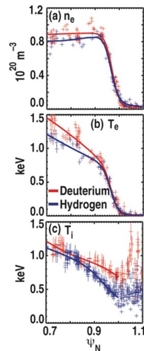
Fig. 2. Comparison of profiles of (a) electron density, (b) electron temperature, (c) ion temperature from D (red) and H (blue) discharges in ITER DEMO configuration.
