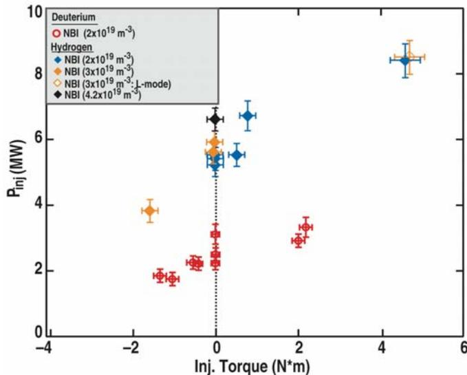
Fig. 1. Injected power required to induce the L-H transition as a function of the injected torque for various target densities. Higher torque data points ( $>3$  Nm) represent all co-NBI discharges in which it was not possible to obtain lower NBI power for the applied torque.
