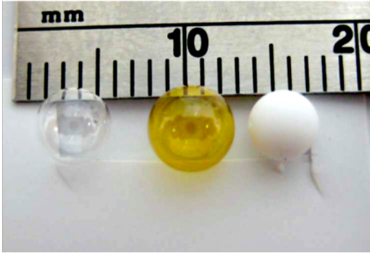
Fig. 5. Three shells: Left, a 4 mm diameter Poly alpha methyl styrene (PAMS) shell with a wall thickness of \sim 35 micron; Center, 5 mm diameter Glow Discharge Polymer (GDP) shell with wall thickness of \sim 20 micron (composition \sim \text{CH}_{1.2} ); Right, a 4 mm diameter Divinyl Benzene (DVB) foam shell with wall thickness of \sim 260 micron and open cell size of \sim 1 micron.
