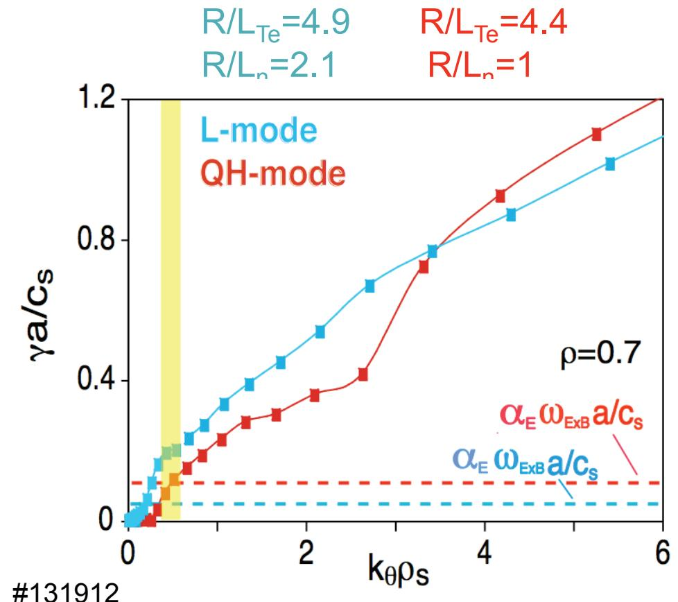
Calculations confirm linear instability in QH-mode for  $r/a > 0.55$  ( $kr_s \geq 0.5$ ).
