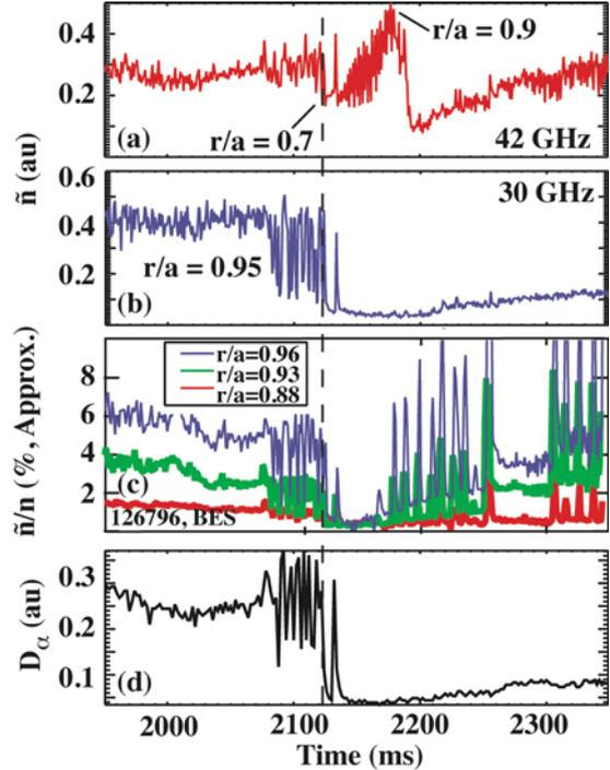
FIG. 4. (a) Backscattered signal ( $f = 42 \text{ GHz}$  with cut-off present, localized as shown,  $k_{\theta} \sim 6 \text{ cm}^{-1}$  ( $r/a \sim 0.7$ , 2100 ms),  $k_{\theta} \sim 4 \text{ cm}^{-1}$  ( $r/a \sim 0.9$ , 2170 ms); (b) 30 GHz ( $r/a = 0.95$ ,  $k_{\theta} \sim 3 \text{ cm}^{-1}$ ); (c) relative density fluctuation level at low wave-number  $k_{\theta} < 3 \text{ cm}^{-1}$  (BES); (d)  $D_{\alpha}$  signal across the L-H transition (dashed line).
