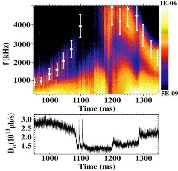
FIG. 6. Doppler spectrum vs time across the L-H transition in a low density QH-mode shot (#131902,  $0.35 \leq r/a \leq 0.8$ ).  $f_{\text{ExB}}$  from CER is indicated by white symbols. Also shown is the  $D_\alpha$  signal indicating the transition timing.
