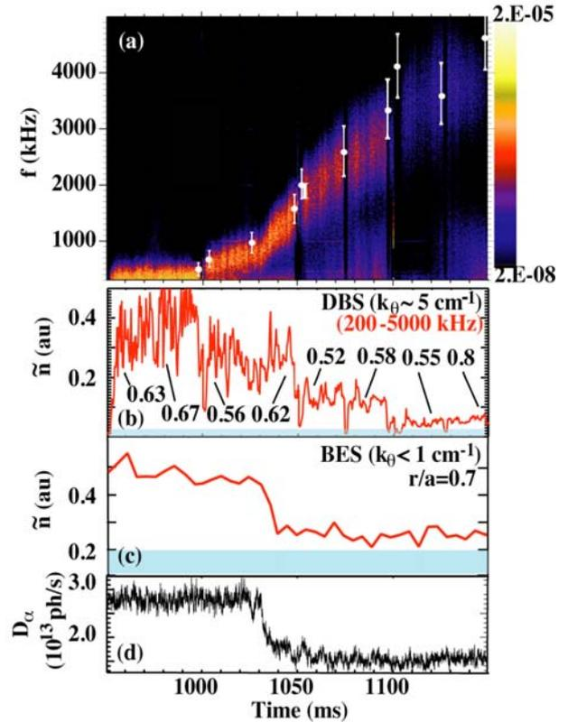
FIG. 7. (a) Doppler spectrum vs time ( $f_{\text{ExB}}$  from CER is indicated by white symbols), (b) intermediate scale fluctuation level ( $0.52 \leq r/a \leq 0.8$  as indicated), (c) low- $k$  ( $< 1 \text{ cm}^{-1}$ ) fluctuation level from BES, and (d)  $D_\alpha$  signal across the L-H transition in a low density QH-mode shot (#131912). The sensitivity/noise level is indicated in (b) and (c).
