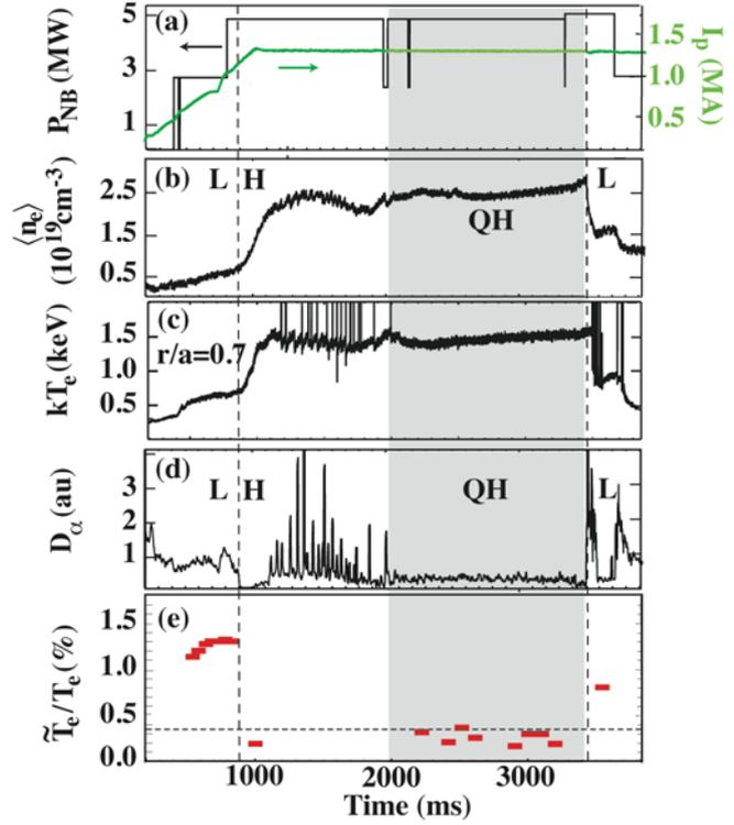
FIG. 1. (a) Neutral beam power and plasma current; (b) line-averaged density; (c) electron temperature at  $r/a=0.7$ ; (d)  $D_\alpha$  line emission intensity; (e) normalized electron temperature fluctuation level ( $r/a=0.7$ ) for shot #125113. L-H and H-L transitions are indicated by vertical dashed lines, the QH-mode phase is shaded.
