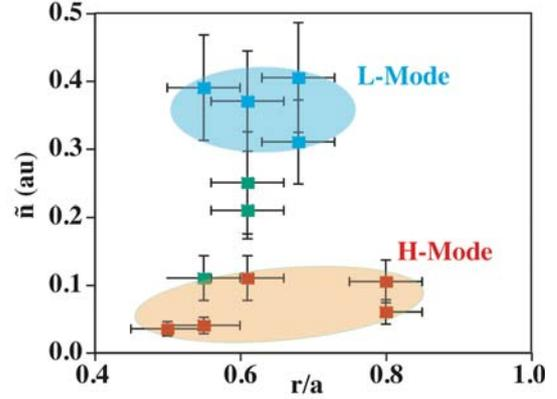
FIG. 8. Measured intermediate-scale fluctuation levels in L- and H-mode (#131912). Data from the L-H transition period are also included (green symbols).
