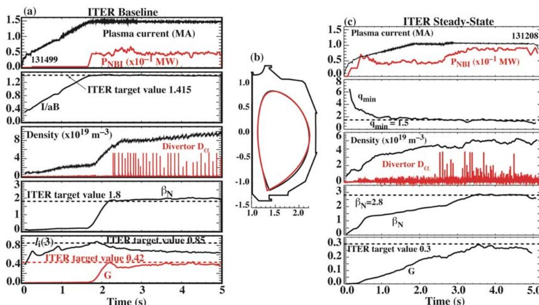
Fig. 1. (a) Key parameters for an ITER baseline scenario demonstration discharge, (b) scaled ITER Scenario 2 plasma shape, preserving aspect ratio of 3.1 (black), and experimental DIII-D shape (red), and (c) key parameters for ITER steady-state scenario demonstration discharge.
