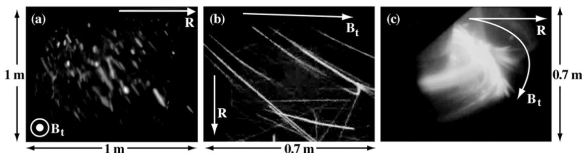
Fig. 1. Dust in DIII-D: (a) dust produced by a disruption (fast camera, tangential view of outboard SOL); (b) dust observed after an entry vent (standard rate camera, looking down in the lower divertor); (c) intentional dust injection into the lower divertor (standard rate camera, tangential view of the lower divertor).
