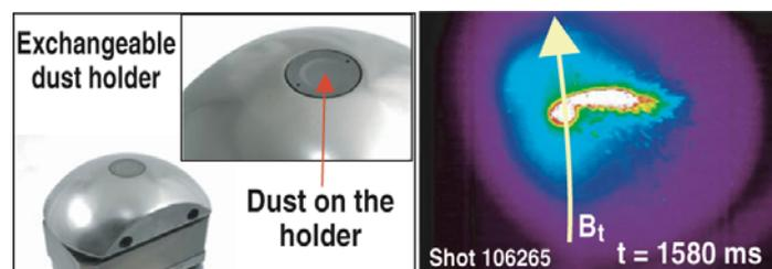
Fig. 2. The dust experiment in TEXTOR: (a) spherical graphite test limiter with exchangeable holder and dust; (b) the launch of dust at the beginning of NBI phase.
